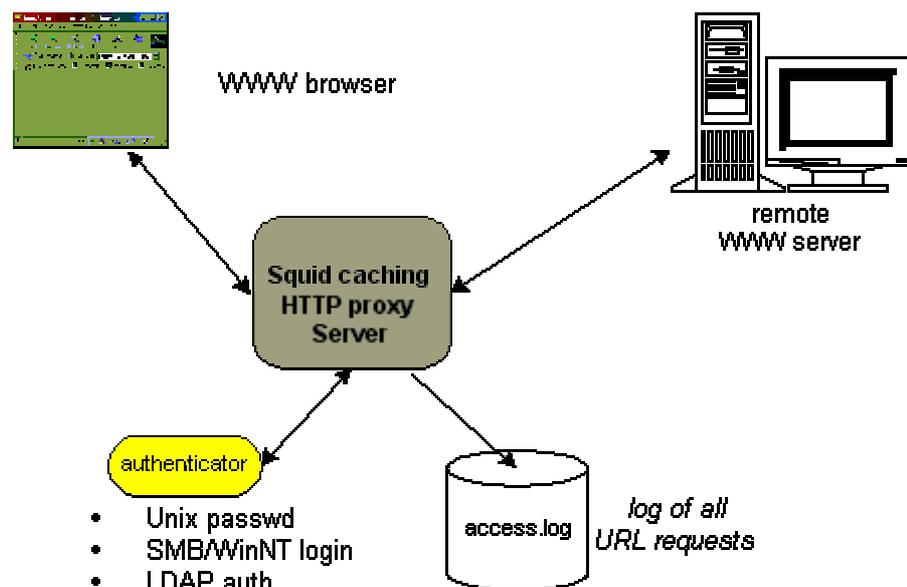
The main reason for using a caching proxy server is to reduce the demand for bandwidth by caching downloaded objects on the server. If a user requests an object that has previously been requested by another user at our site, then the proxy server can deliver the object directly to the
