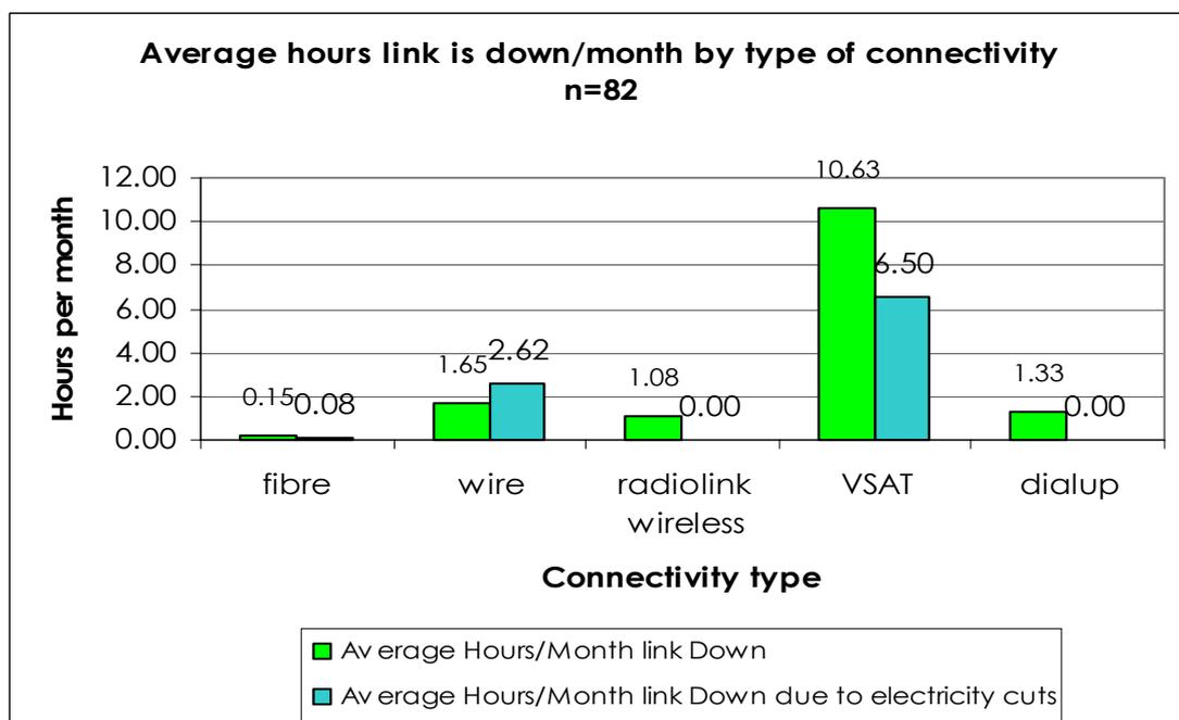
The results indicate that VSATs have a higher rate of failure, with 10.63 hours per month, than other links, with fibre having the lowest rate of failure of 0.15 hours per month. It appears that, where electricity cuts are a problem, VSAT and wire are affected most. The implications of these findings is that VSAT solutions appear to be a more difficult technical solution for many institutions, and additional support is likely to be needed when implementing this solution.
